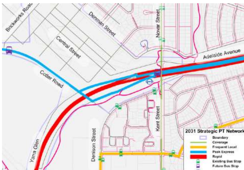
Fig. 16 Proposed Bus Stop Adelaide Avenue (SMEC 2015) with buses needing to reverse plus loss of T2 lanes
